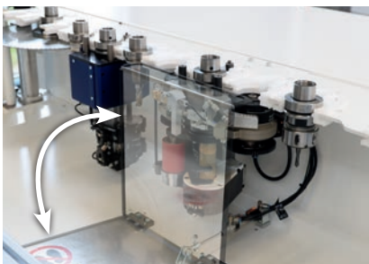
Electrical interface for the side linear changer for parallel heating of the edge banding unit.
