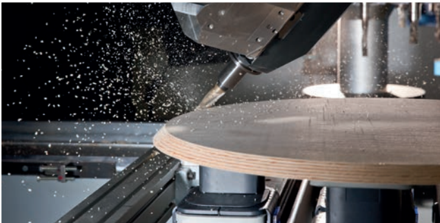
Chamfer cutting on a table top
