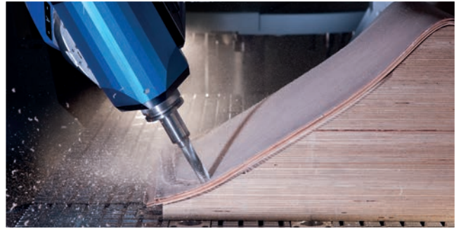
Routing of shaped wood
