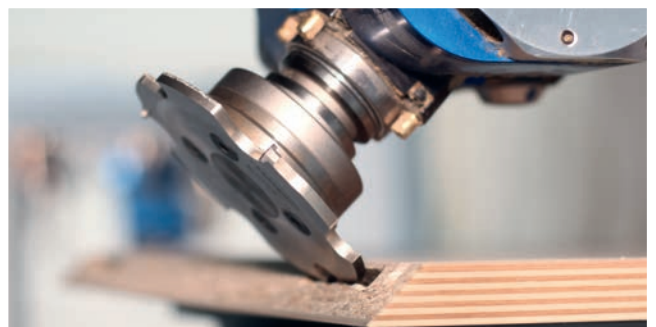
Cutting recesses for connecting fittings
