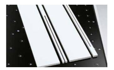
In manual operation, the cut-out feature allows you to produce even cut-outs and insertion grooves immediately - for example, for doors or kitchen sinks.
